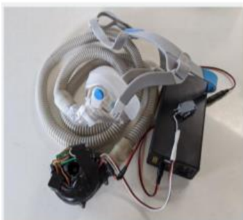
Arduino based ventilator system from Italy Research firm
