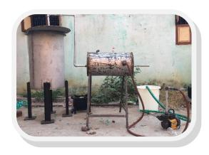
Pyrolysis is a thermochemical decomposition of organic material at elevated temperatures in the absence of oxygen .
