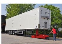
rolling trolley. The Verhagen Leiden V-Move Trailer Mover XXL pairs a 4kW electric motor with a 36-volt 245Am battery pack to provide the necessary pulling power, with Continental tires delivering the
