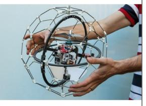
absorbed by the cage alone, with an onboard electronic stabilizing mechanism automatically leveling the assembly, so it can quickly continue flying even after running into an obstacle. That way, the remote pilot doesn't have to bother maneuvering carefully when flying the machine indoors, allowing them to survey the area at a much quicker pace. And when it comes to search and rescue, a
