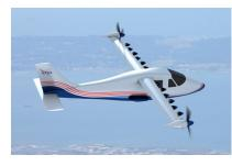
became the first to break the speed of sound. The innovation that's been synonymous with the designation continues with the agency's first X-plane in over a decade: the NASA X-57 Maxwell, the first one to rely exclusively on electric motors for power.
