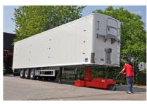
on a rolling trolley. The Verhagen Leiden V -Move Trailer Mover XXL pairs a 4kW electric motor with a 36-volt 245Am battery pack to provide the necessary pulling power, with Continental tires delivering the
