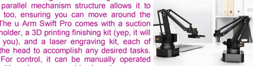
either via mouse-and-keyboard or a companion mobile app, as well as programmed using a graphical interface based on Blockly. It can also learn movements by physically moving the arm, as it can remember motion sequences and repeat it when triggered Do note, it handles maximum payloads of just 1.1 pounds, so while it can carry a brush and paint your walls, you won't be able to use it to hold your power tools in the workshop. (www.coolthings.com)
