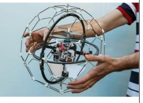
absorbed by the cage alone, with an onboard electronic stabilizing mechanism automatically leveling the assembly, so it can quickly continue flying even after running into an obstacle. That way, the remote pilot doesn't have to bother maneuvering carefully when flying the machine indoors, allowing them to survey the area at a much quicker pace. And when it comes to search and rescue, a
