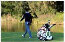
certain distance, you can also control it manually. The remote is good for up to 50 meters, so you can send it far off if you suspect that the droid is the cause of your recent spate of bad luck. Features include downhill braking (it will pace itself going downhill when it notices you're doing the same), an integrated stabilizer, and high-grip V3 wheels.
